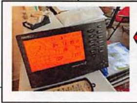
This is the console, a blinking X in the bottom right of the console screen indicates that it is collecting data every 4-5 mins.
